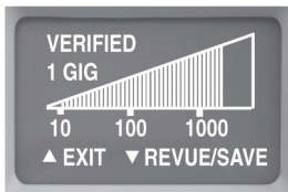
Figure 6-19. LPV Level 2 final screen (when you see this screen, Level 2 is completed and available for review).
